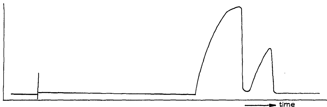
Fig. 4. Separation of 0.5 ml decalin ( trans and cis ) on 6 m coiled glass column, diameter 9 mm, filled with 30% SE 30 on Chromosorb P with hydrogen as carrier gas.
